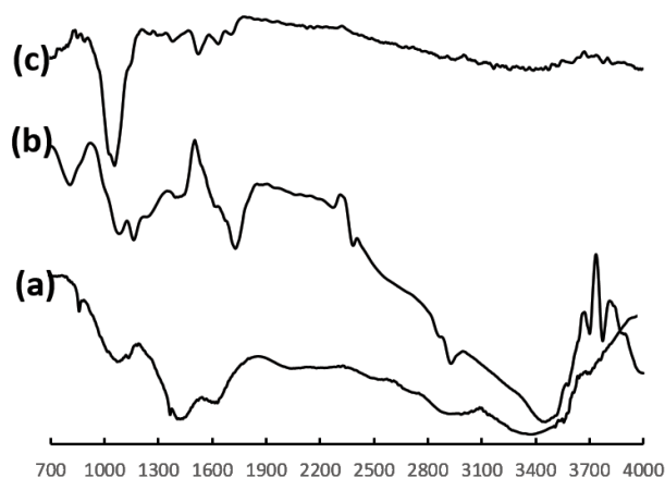
Fig. 1. FTIR analysis of composite (a) chitosan, (b) composite C-1, and (c) composite C-4.
