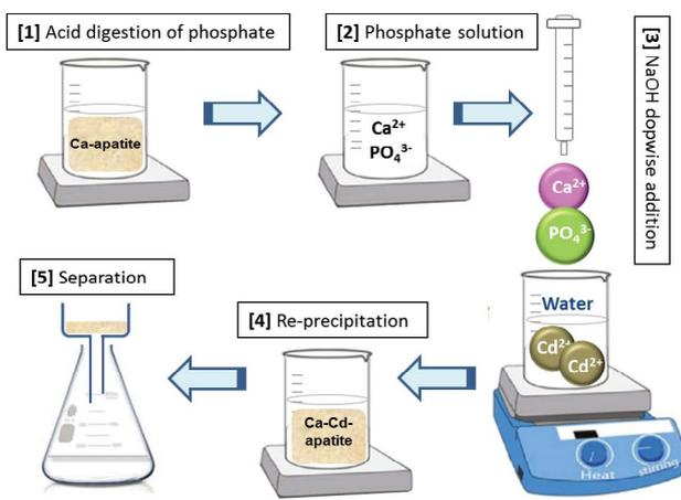
Fig. 1. Schematic illustration of  $\text{Cd}^{2+}$  neutralization in Cd-contaminated water through acid digestion of animal waste bones and NaOH-assisted precipitation of Ca-Cd-phosphate apatites.
