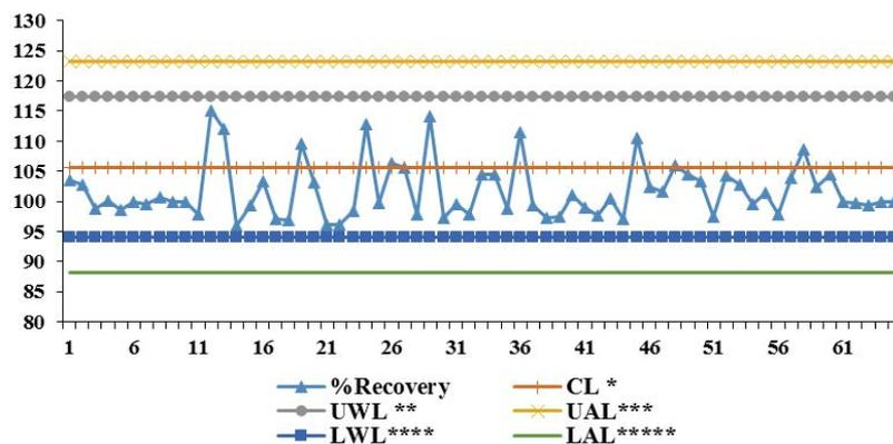
Fig. 6. Recycling evaluation of 2,4-D in real samples for all sampling cases in the range of studied time via performance parameters of enriched binary laboratory matrix (sample volume: 49.5 mL; the standard added volume of 2,4-D: 0.5 ppb; added concentration of 2,4-D: 1,000 ppb). \*Control levels; \*\*upper warning limits; \*\*\*upper action limits; \*\*\*\*upper warning limits; \*\*\*\*\*lower action limits.
