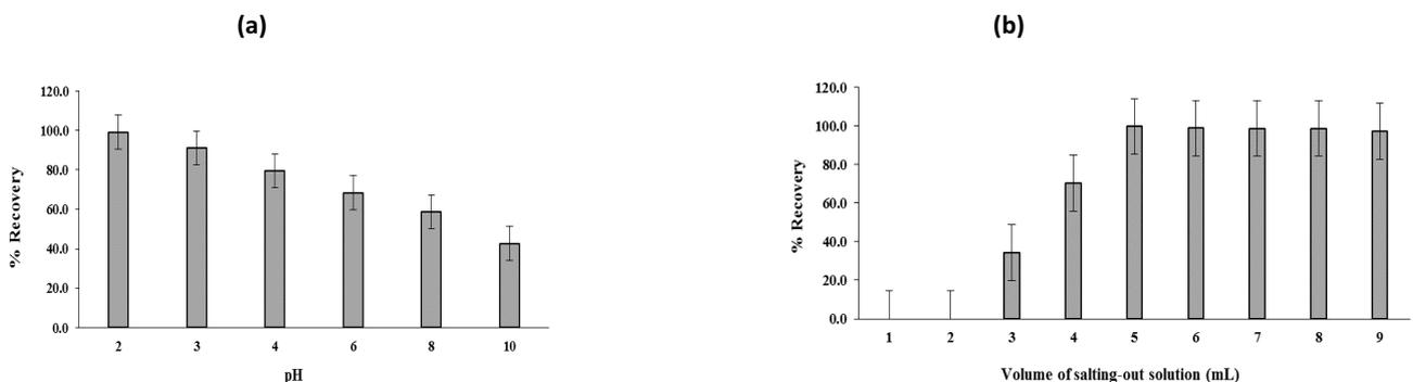
Fig. 2. (a) Effect of solution pH on extraction efficiency of 2,4-D (SALLE conditions: extraction solvent, ACN, 1 mL; sample volume, 4 mL; volume of salting-out solution, 6 mL NaCl (%5 (w/v))) and (b) effect of salting-out solution volume on extraction efficiency of 2,4-D (SALLE conditions: extraction solvent, ACN, 1 mL; sample volume, 4 mL; pH = 2; salting-out solution, NaCl (%5 (w/v))).
