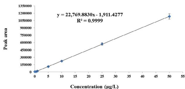
Fig. 3. Calibration curve of 2,4-D at different concentrations (0.01 to 50 µg/L).
