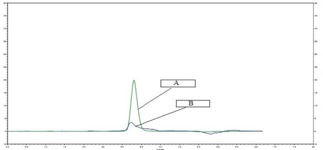
Fig. 5. Typical representative chromatogram of (A) real sample with unspike 2,4-D and (B) real sample with spiked 2,4-D (HPLC operating conditions: mobile phase: methanol–water–acetic acid (80:19.5:0.5, v/v); flow rate 1.5 mL/min; analytical column C18; UV detection at wavelength = 280 nm; injection volume = 20  $\mu$ L).
