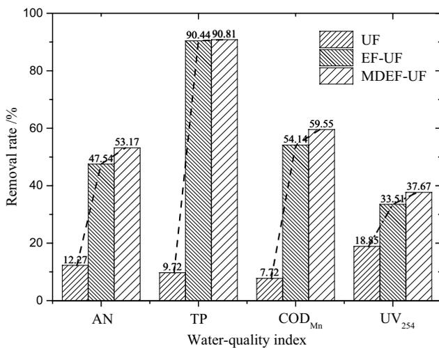
Fig. 3. Comparison of the removal rate using three types of treatment processes.
