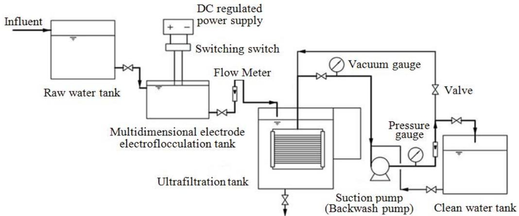
Fig. 1. Flow chart of the combination multidimensional electrode electro-flocculation and submerged ultrafiltration devices.
