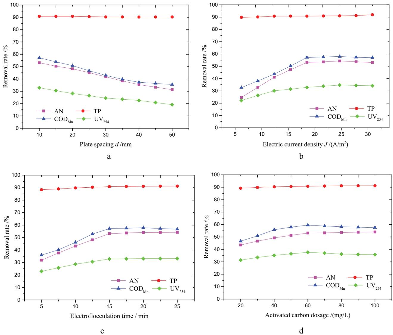
Fig. 2. Ammonia nitrogen, TP,  $COD_{Mn}$  and  $UV_{254}$  removal rates as a function of (a) plate spacing, (b) electric current density, (c) electro-flocculation time, and (d) activated carbon dosage.
