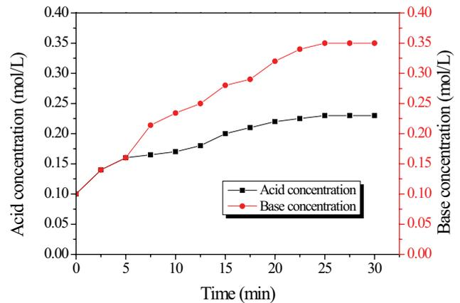
Fig. 4. Concentration of acid and base generated from pesticide wastewater by BMED.
