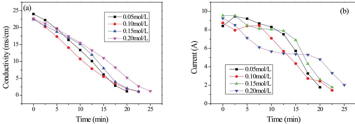
Fig. 8. Conductivity (a) and current density (b) of the BMED process with different initial base and acid concentrations.
