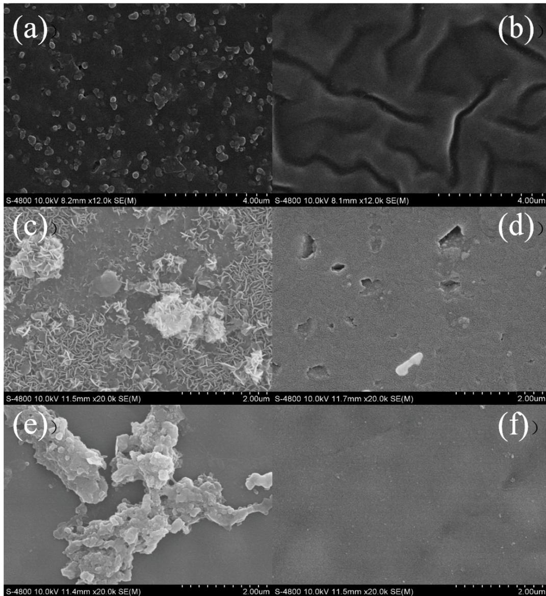
Fig. 11. SEM images of BM, CEM, and AEM in the treatment of pesticide wastewater by BMED process and after the backwash. (Cation side (a) and anion side (b), polluted CEM (c), CEM after backwash (d), polluted AEM (e), and AEM after backwash (f).
