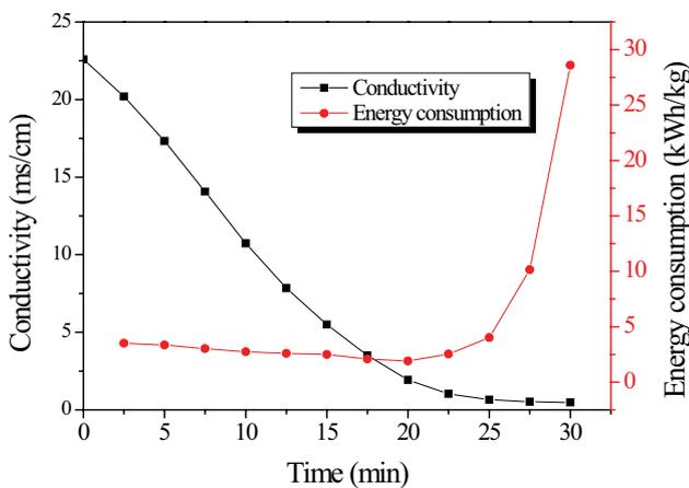
Fig. 3. Relation between the conductivity and energy consumption of the pesticide wastewater at the end of the BMED process at 30 V.
