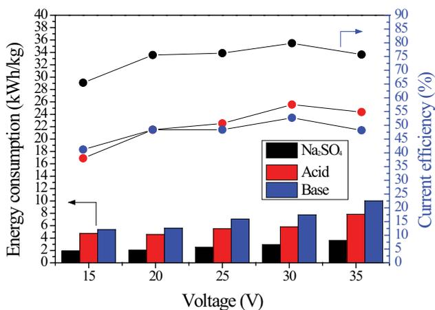
Fig. 7. Current efficiency and energy consumption of BMED process with different operational voltages.
