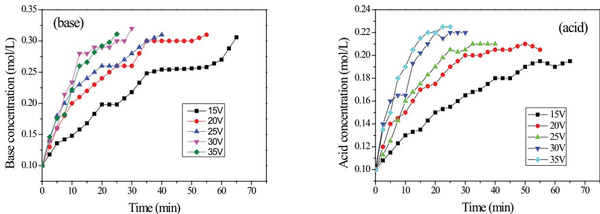
Fig. 6. Concentrations of acid and base generated by BMED process at different voltages with initial acid/base concentration 0.1 mol/L.
