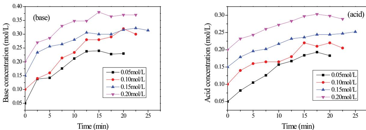
Fig. 9. Concentrations of acid and base generated by BMED process at different initial acid/base concentrations with voltage 30 V.
