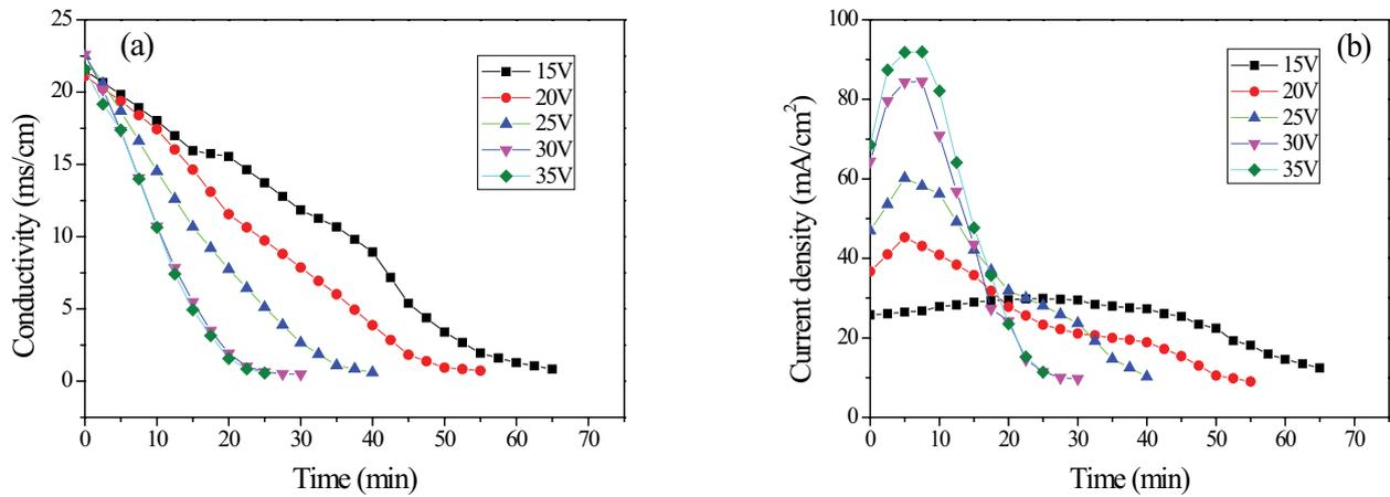
Fig. 5. Conductivity (a) and current density (b) of the BMED process under different operational voltages.
