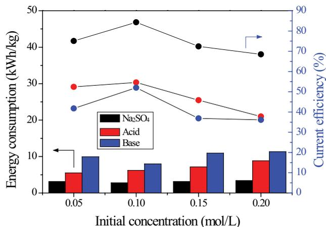
Fig. 10. Current efficiency and energy consumption of BMED process with different initial concentrations of acid and base.
