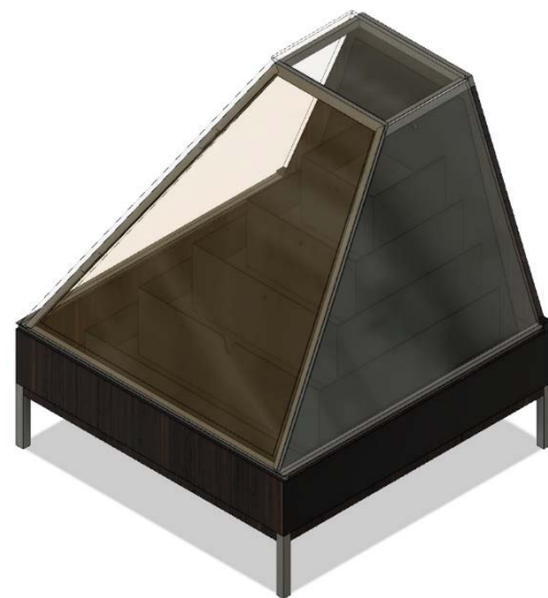
Fig. 1. Three-dimensional view of the pyramid still with chamber step-wise design.
