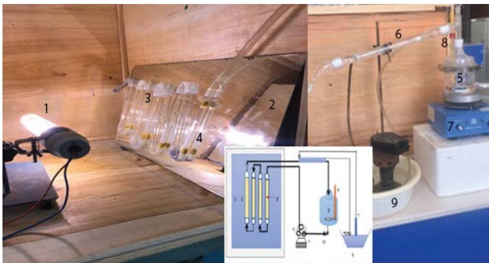
Fig. 3. Schematic diagram of the pilot: (1) visible light, (2) mirror, (3) photoreactor, (4) TiO 2 -P/SPA catalyst coated on glass microspheres, (5) reactor containing naphthalene solution, (6) condenser, (7) magnetic stirrer, (8) thermometer, and (9) cooler pump and cold water tank.
