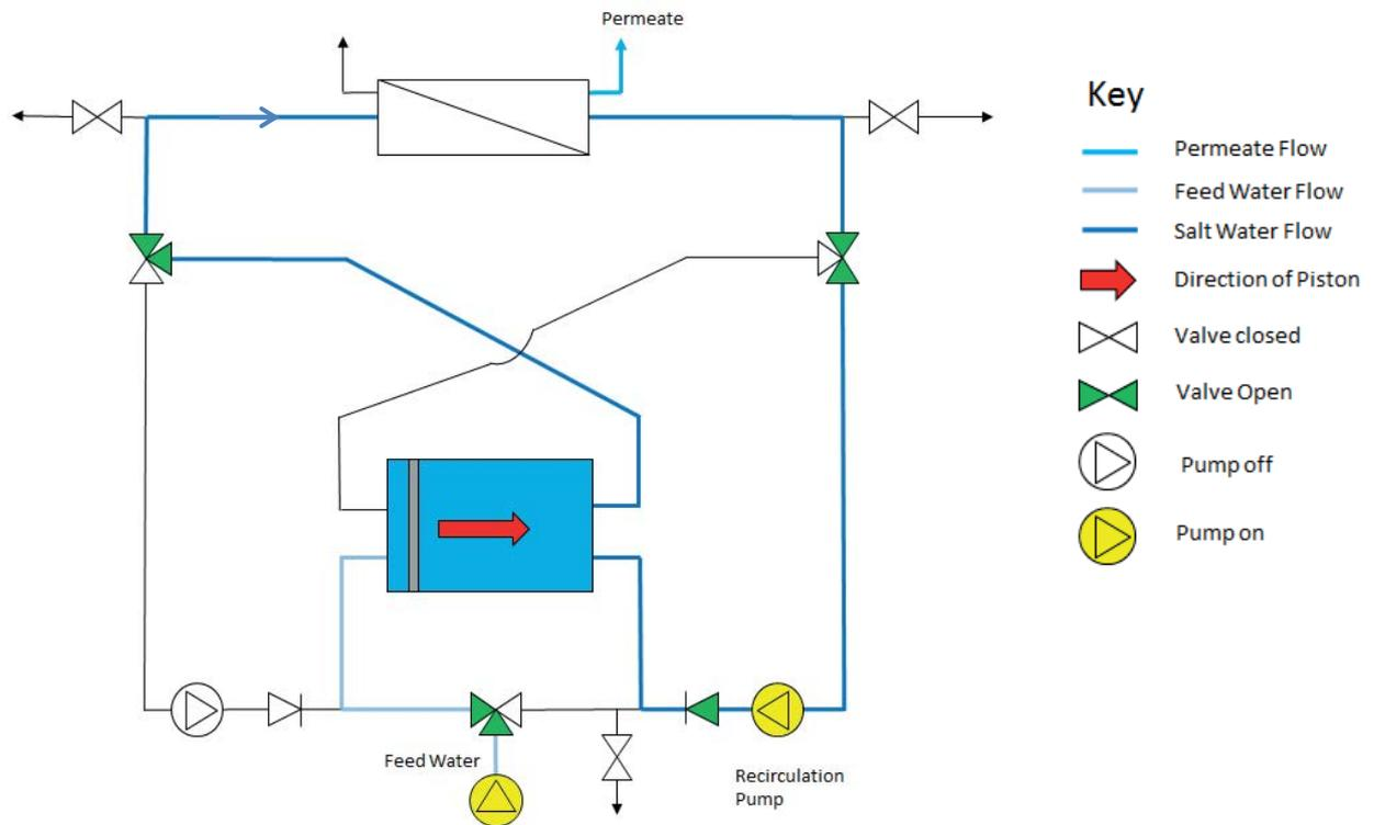
Fig. 10. Stage 1; pressurization (first time).
