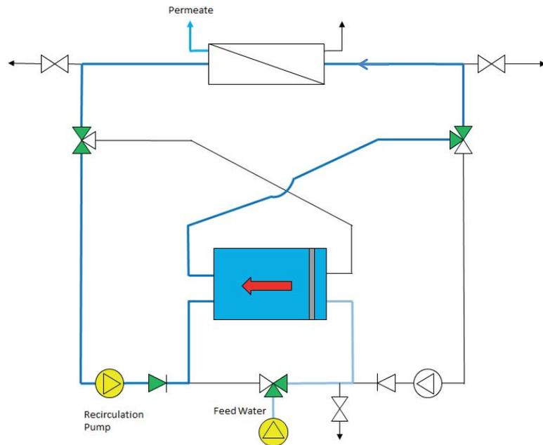
Fig. 12. Stage 3; pressurization (second time).
