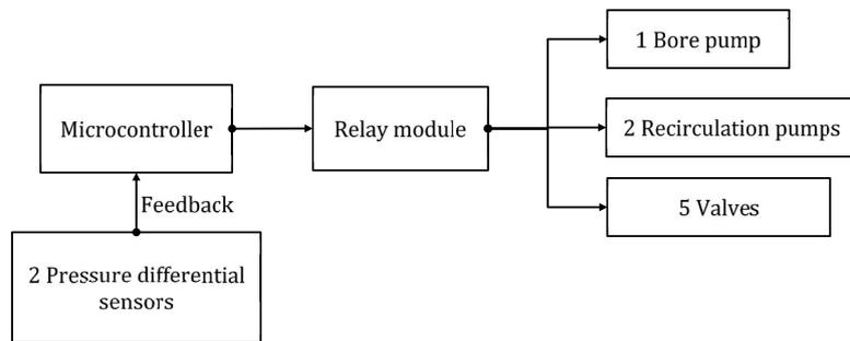
Fig. 14. Electric control of the system, using Arduino.
