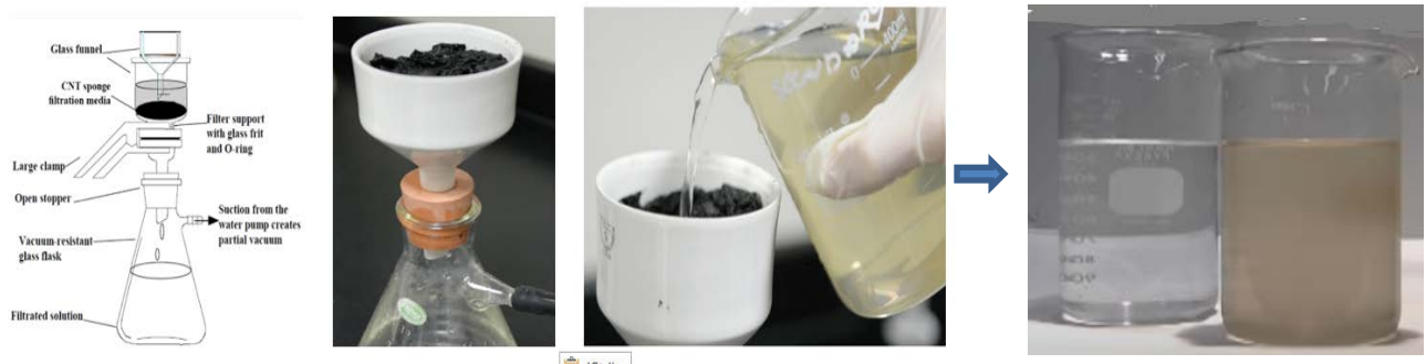
Fig. 2. Vacuum filtration of raw sewage using CNT sponge as filtering media.
