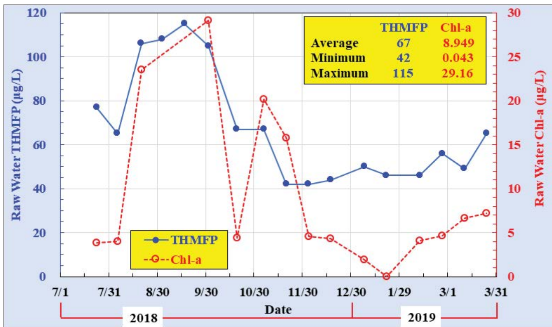
Fig. 7. Variations of the THMFP and the Chl-a of the feed (measured by BWQI).
