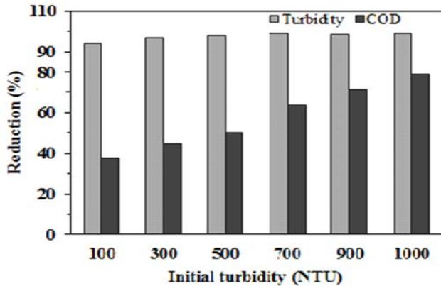
Fig. 4. Influence of the variation of the initial turbidity on the efficiency of the EC.
