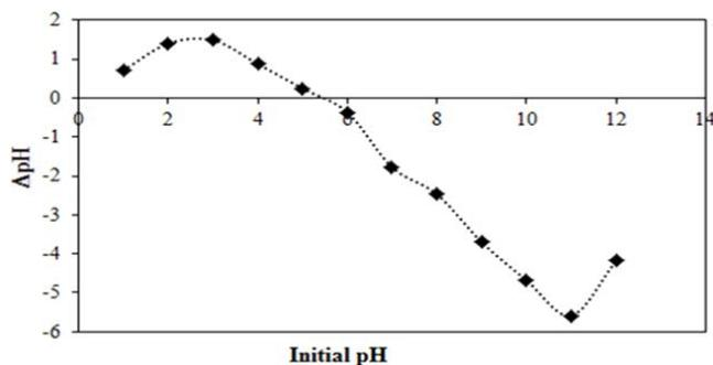
Fig. 11. Point of zero charges of OFIP.
