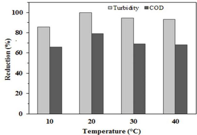
Fig. 5. Influence of the variation of the initial temperature on the efficiency of the EC.
