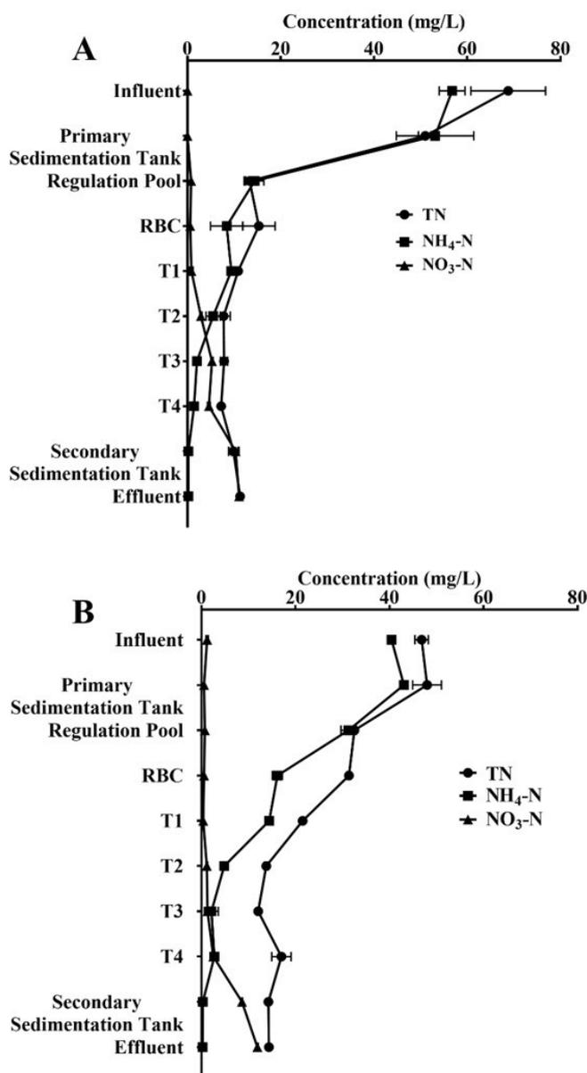
Fig. 2. Total nitrogen (TN), ammonium (NH<sub>4</sub>-N), and nitrate (NO<sub>3</sub>-N) in different treatment units; (A) July and (B) December of 2016. Scale bars represent the standard deviation of three replicates.
