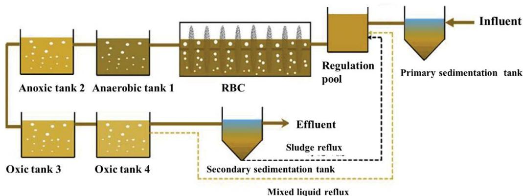
Fig. 1. Diagram of treatment units and processes used in the WWTP system.
