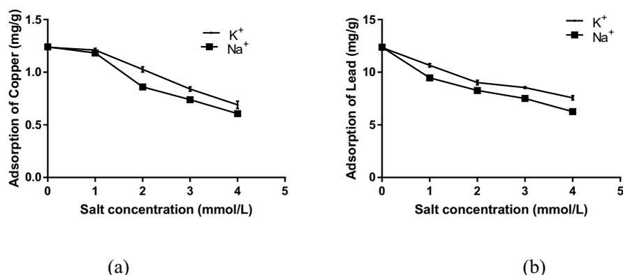
Fig. 4. Effects of K<sup>+</sup> and Na<sup>+</sup> on the adsorption of copper (a) and lead (b) by R12.
