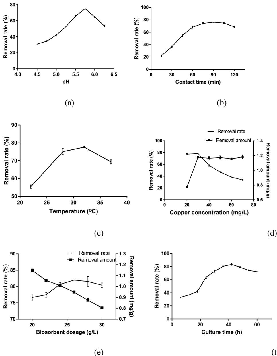
Fig. 2. Effects of adsorption parameters on the removal of  $\text{Cu}^{2+}$  by R12. Effects of (a) pH, (b) contact time, (c) temperature, (d) initial copper concentration, (e) biosorbent biomass, and (f) culture phase on the removal of  $\text{Cu}^{2+}$  by R12.
