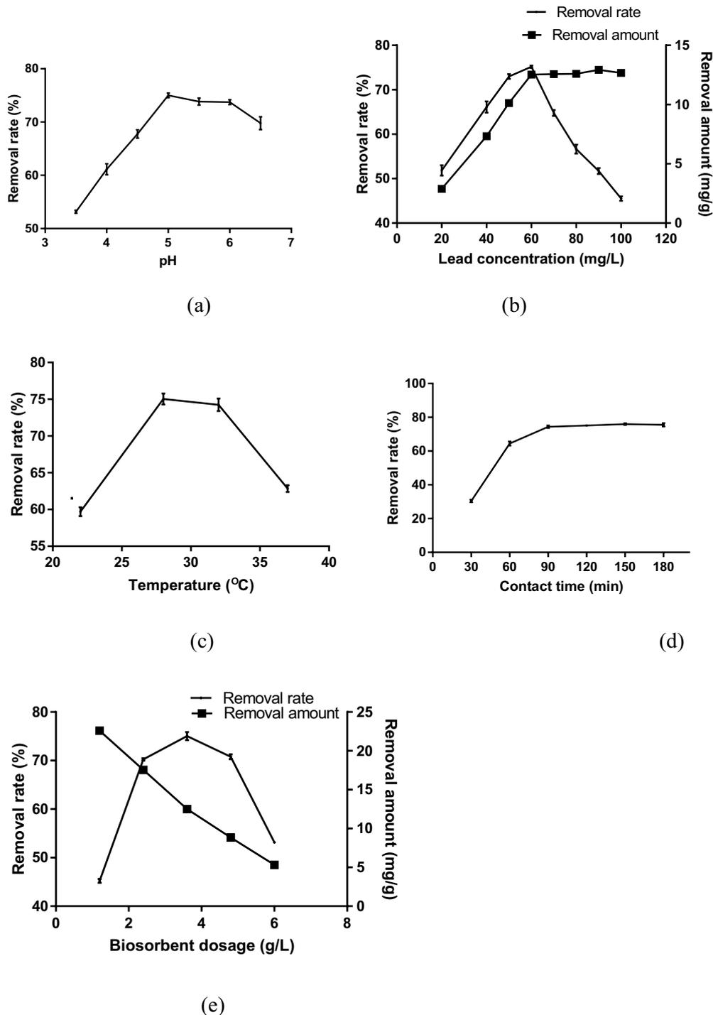
Fig. 3. Effect of adsorption parameters on the removal of Pb<sup>2+</sup> by R12. Effect of pH (a), initial lead concentration (b), temperature (c), contact time (d), and biosorbent dosage (e) on the removal of Pb<sup>2+</sup> by R12.
