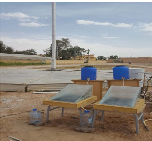
Fig. 4. The photo of the coupled devices solar tower-solar still and the witness.
