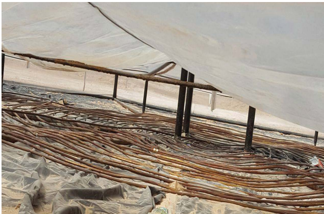
Fig. 3. The photo of the serpentine copper tube.
