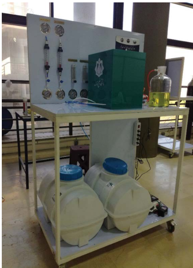
Fig. 1. Integrated system of ED-RED on pilot scale.
