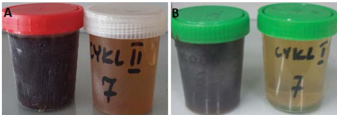
Fig. 3. Difference in colour removal for single-step continuous process (for the ratio 1:2:1 – A and for ratio 1:2.5:1.25 – B).
