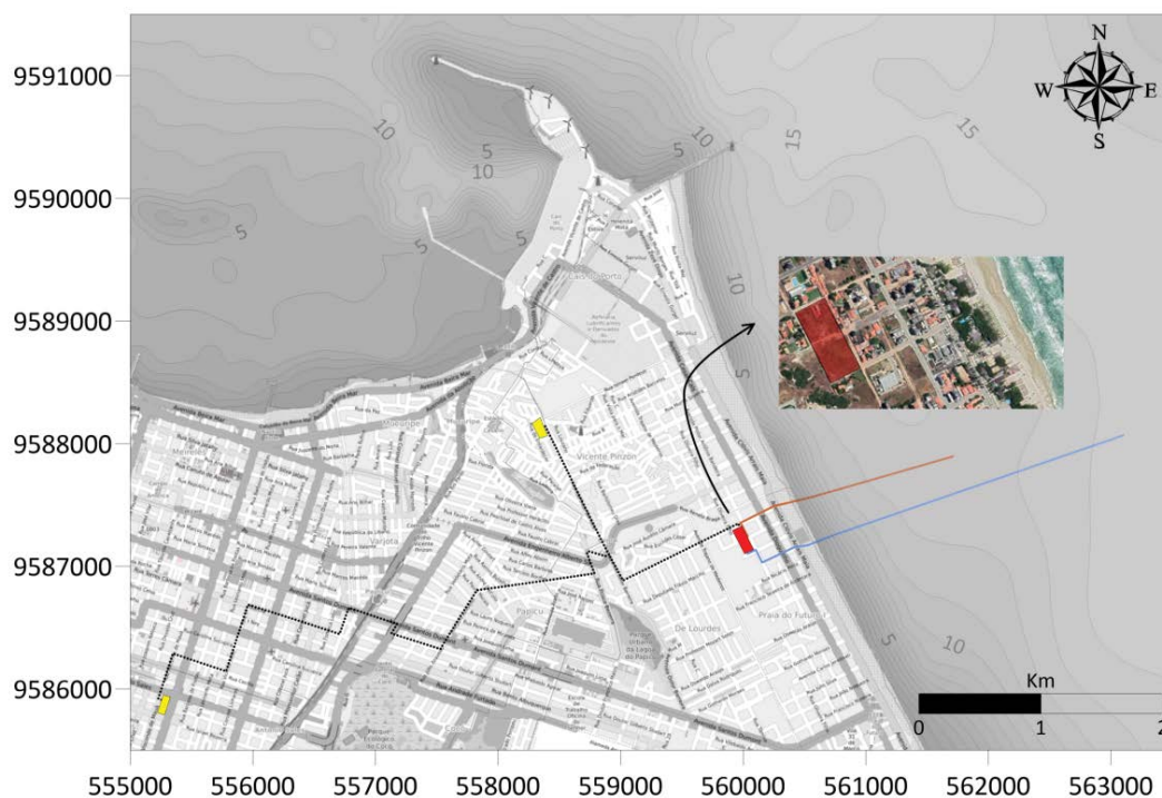
Fig. 1. Map showing the desalination plant, its outfall position (orange line) and water intake (blue).
