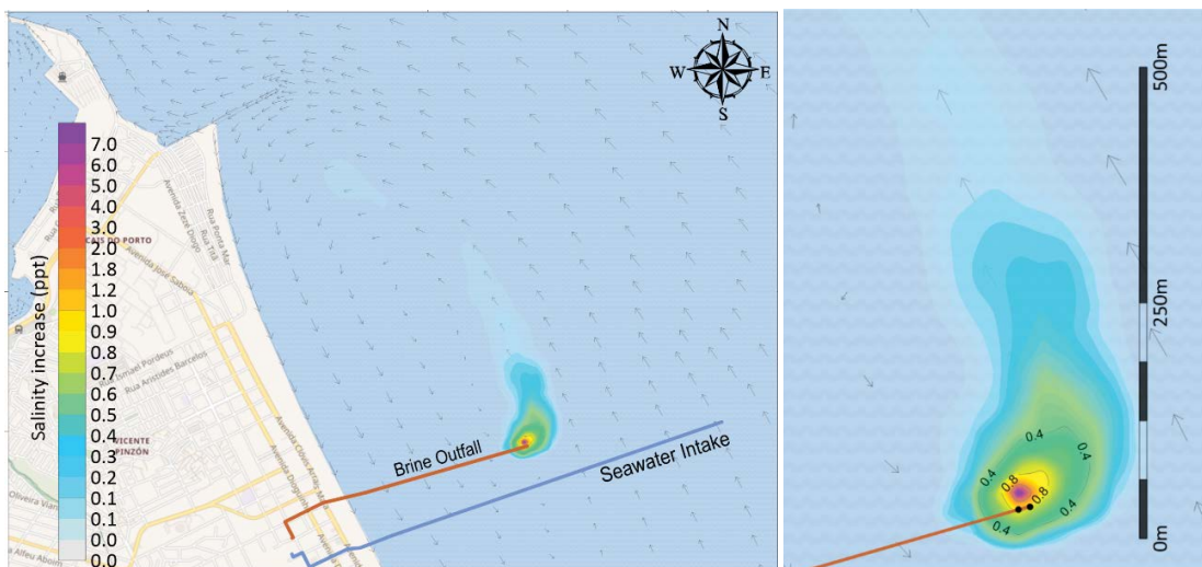
Fig. 10. Increase in salinity (ppt) due to saline concentrate disposal by the outfall, in a given period of April.
