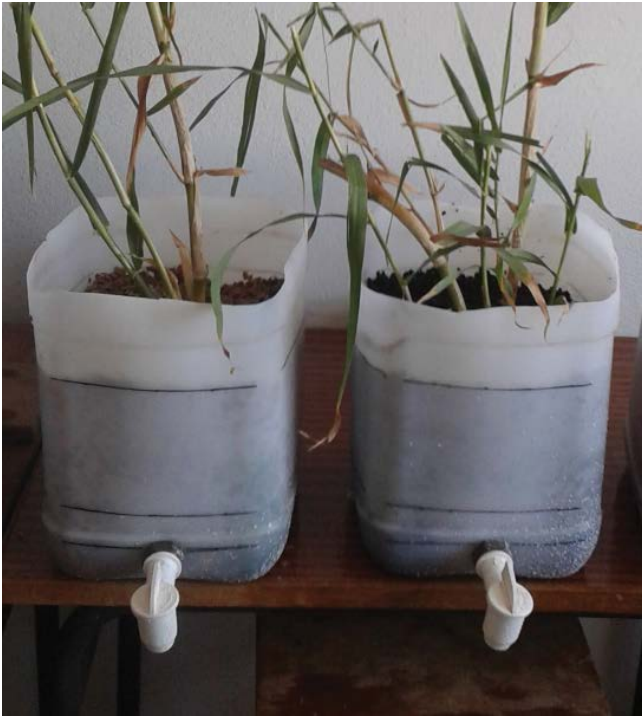
Fig. 2. Laboratory scale prototype of the vertical flow filter with reeds.
