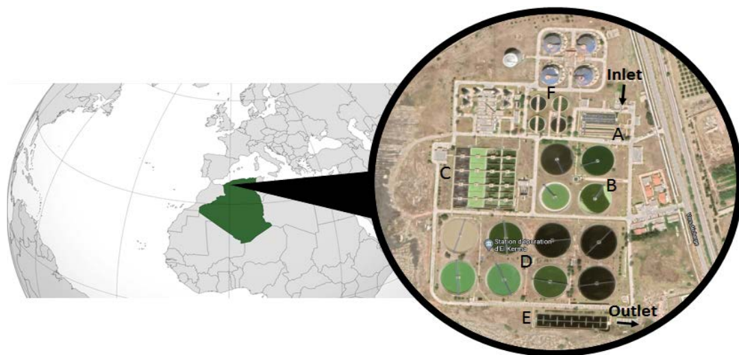
Fig. 1. The Oran wastewater treatment plant localization (latitude: 35.60, longitude: -0.58). A: Preliminary treatment; B: Primary settling; C: Biological treatment; D: Clarification; E: Disinfection; F: Sludge treatment.
