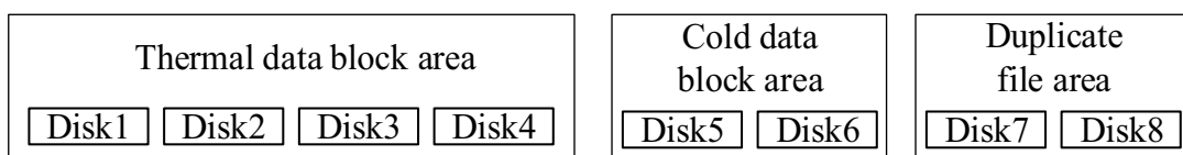
Fig. 3. A storage structure of data classification.
