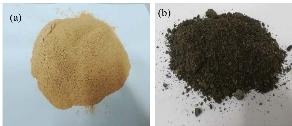
Fig. 1. Sample of testing material (a) kaolin powder and (b) bottom ash.
