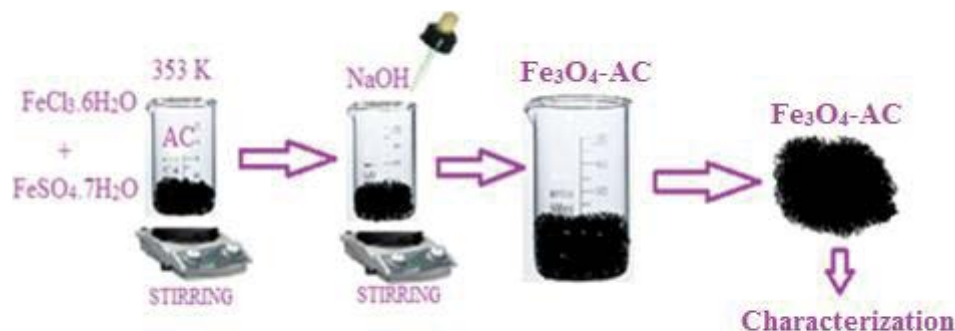
Fig. 1. The synthesis schema of the \text{Fe}_3\text{O}_4 -AC adsorbent.
