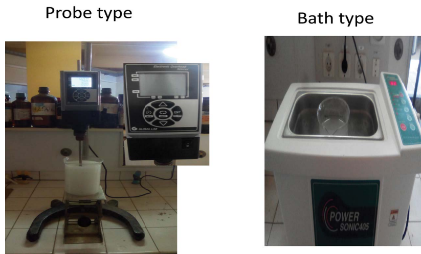
Fig. 5. Nanofluid stirring method: probe-type, ultrasonic bath ultrasound.
