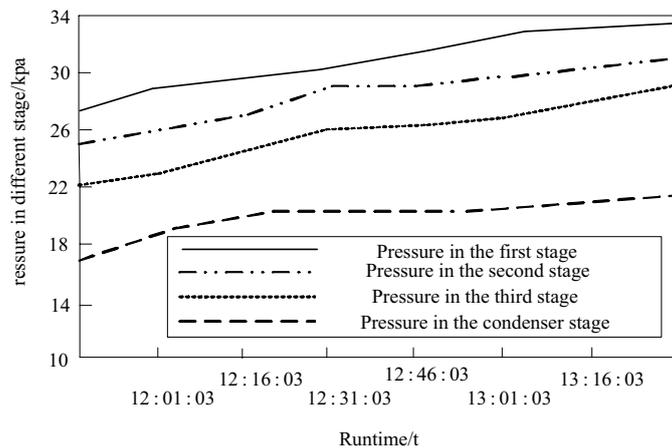
Fig. 5. Pressure transient performance of seawater desalination plant.
