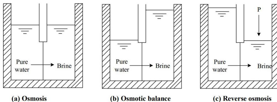
Fig. 1. Information fusion based reverse osmosis principle.
