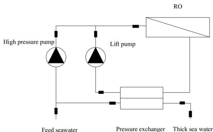
Fig. 4. Typical parallel reverse osmosis and functional exchange energy recovery process.
