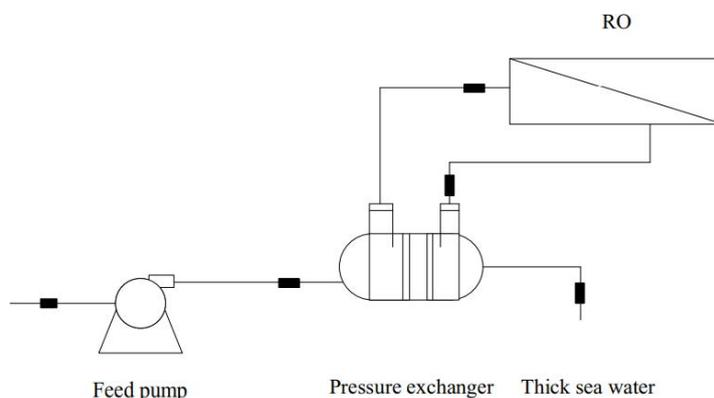
Fig. 3. Typical reverse osmosis and hydraulic turbine energy recovery process in series.
