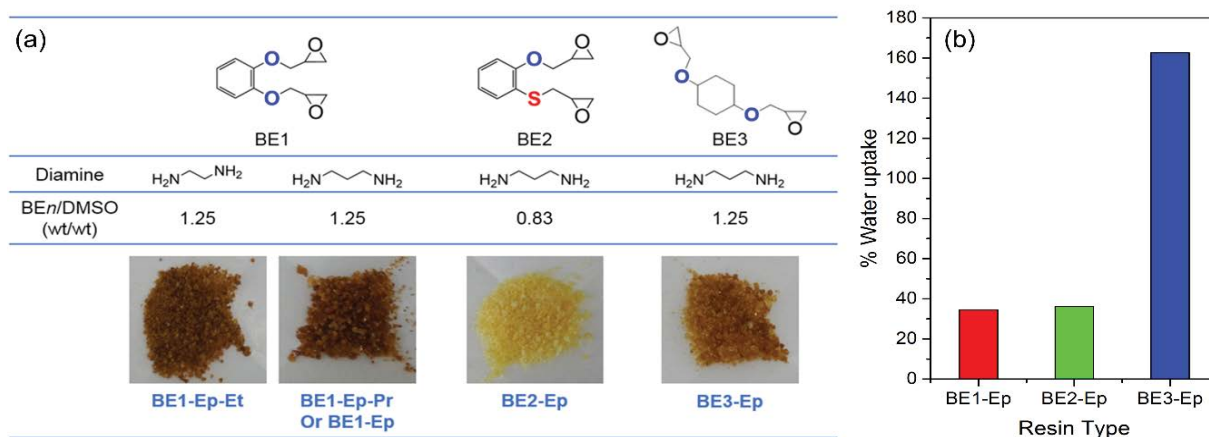
Fig. 2. (a) Epoxy resins produced as solid adsorbents by controlling the amount of DMSO solvent and (b) swelling test of the resins through % water uptake.
