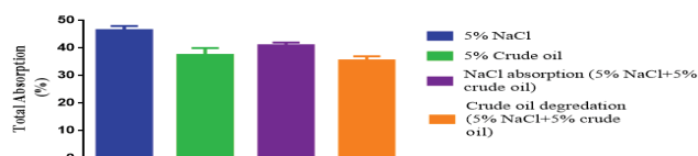
Fig. 11. Effect of NaCl and oil absorption on each other; Regarding the total absorption rate, there is no difference between the NaCl and crude oil absorptions alone or simultaneously. One-way ANOVA was used combined with Tukey's post hoc test. Data are represented as mean ± scanning electron microscopy.
