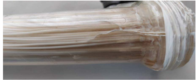
Fig. 13. Photograph of cracked shell.
