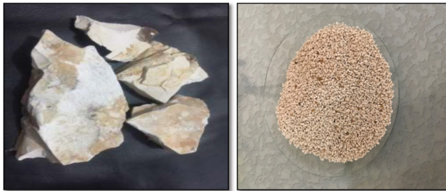
Fig. 5. Porcelanite before and after cracking.
