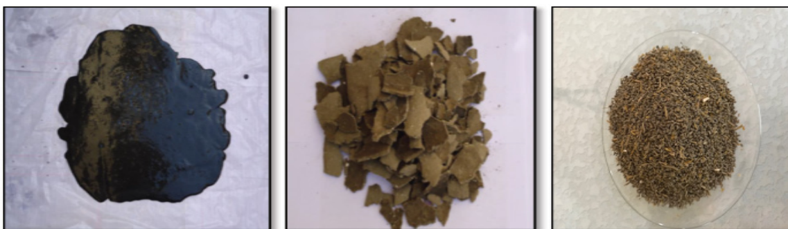
Fig. 6. Anaerobic sludge during drying, flocks of drying dead anaerobic sludge, and after grinding.
