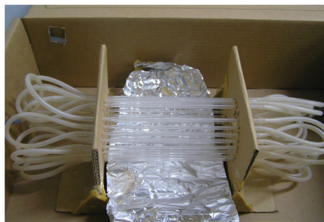
Fig. 1. Schematic diagram of the reactor set-up designed to photocatalytically assess the catalyst supported in the quartz glass tubes.
