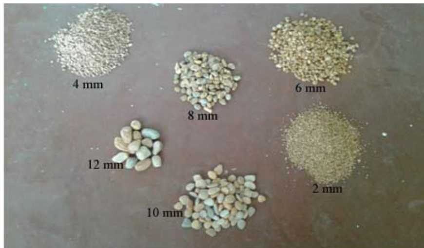
Fig. 2. Schematic diagram of the different diameter pebbles used in the still.
