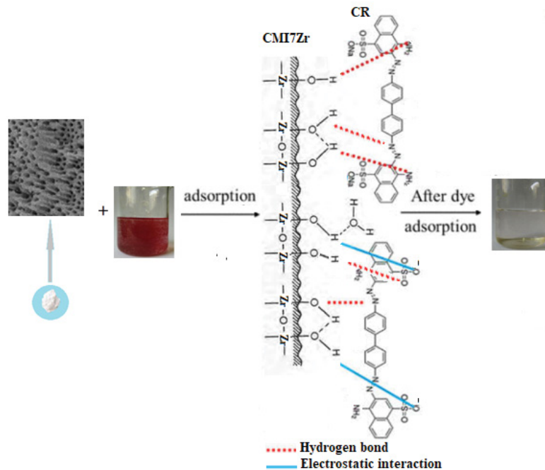
Fig. 16. Proposed schematic adsorption mechanism of zirconia oxide (CMI7Zr).
