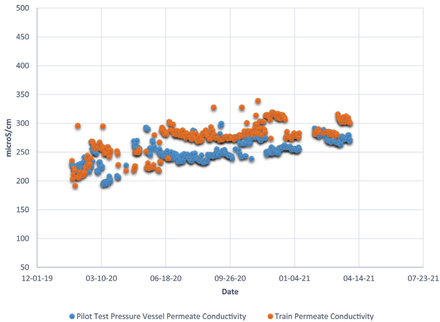
Fig. 7. Train permeate conductivity and pilot permeate conductivity.
