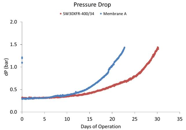
Fig. 12. Normalized pressure drop evolution for FilmTec™ SW30XFR-400/34.
