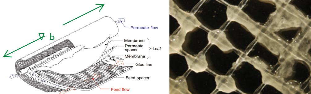
Fig. 1. Reverse osmosis element configuration (a) and biofouled feed spacer (b).
