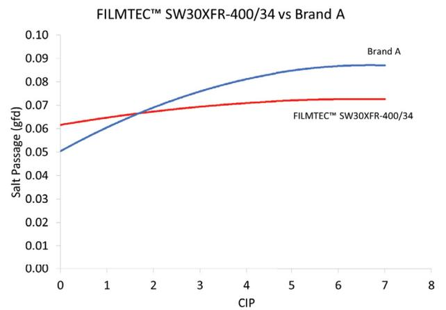
Fig. 13. Durability study comparing FilmTec™ SW30XFR-400/34 vs. another manufacturer named Brand A.
