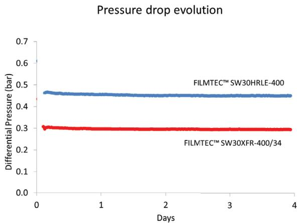
Fig. 11. Pressure drop evolution of FilmTec™ SW30HRLE-400 vs. SW30XFR-400/34.
