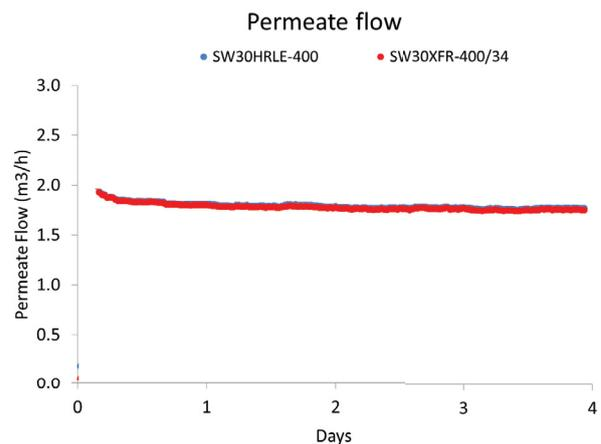
Fig. 9. Permeate flow evolution over time of FilmTec™ SW30HRLE-400 vs. SW30XFR-400/34.
