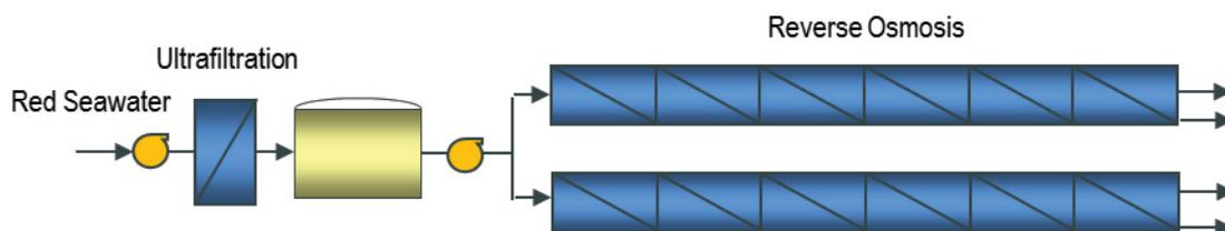
Fig. 5. The DuPont’s MEIC Water Solutions pilot plant scheme, fed by Red Seawater.
