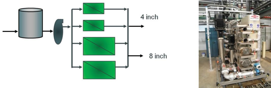
Fig. 2. Diagram and picture of the single element testing plant.
