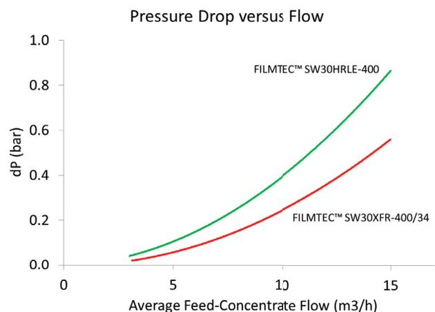
Fig. 8. Pressure drop comparison of new FilmTec™ SW30XFR-400/34 membrane vs. the previous generation SW30HRLE-400.
