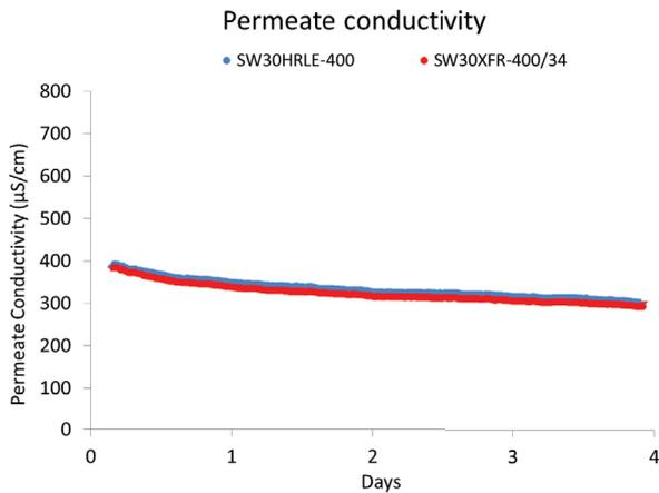
Fig. 10. Permeate conductivity evolution of FilmTec™ SW30HRLE-400 vs. SW30XFR-400/34.
