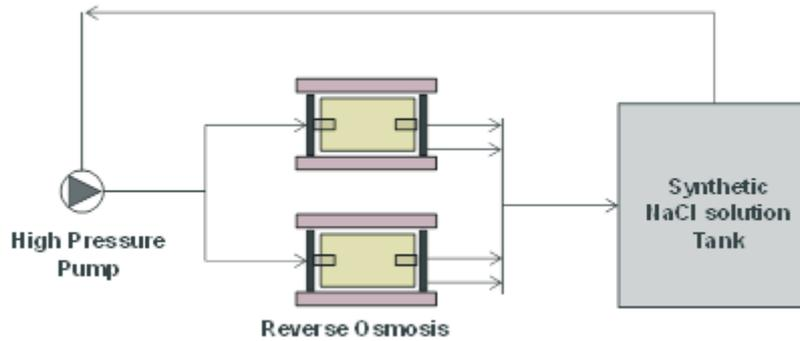
Fig. 7. Durability study pilot plant.
