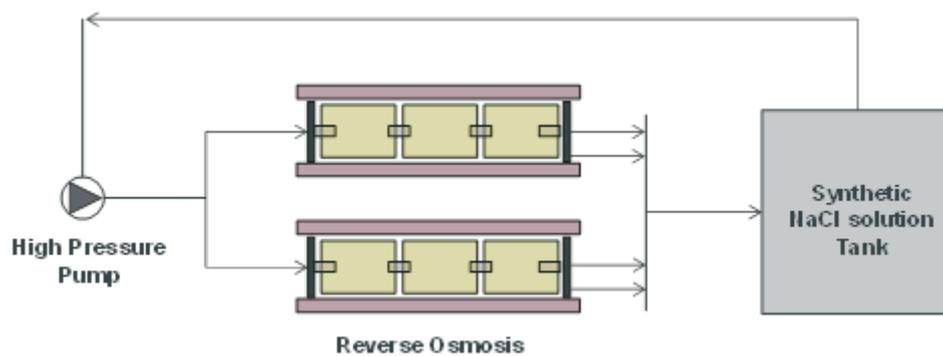
Fig. 3. Synthetic seawater pilot plant schematic.
