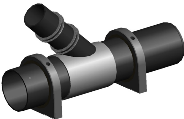
Fig. 12. Diffuser installed in Skikda desalination plant (Algeria).
