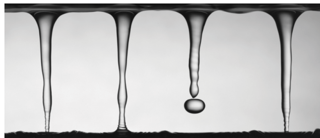
Fig. 10. Drop-column flow pattern.
