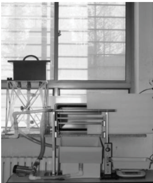
Fig. 2. Horizontal tube falling film flow experimental platform.
