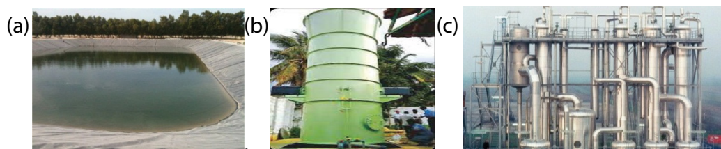
Fig. 4. (a) Solar evaporation, (b) low-cost evaporator and (c) multiple effect evaporator.
