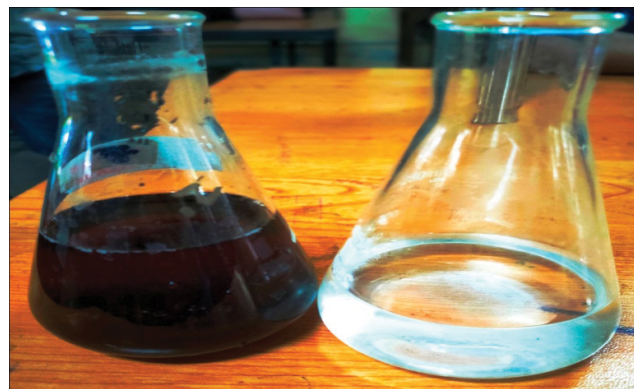
Fig. 6. Coconut husk retting water before and after evaporation.
