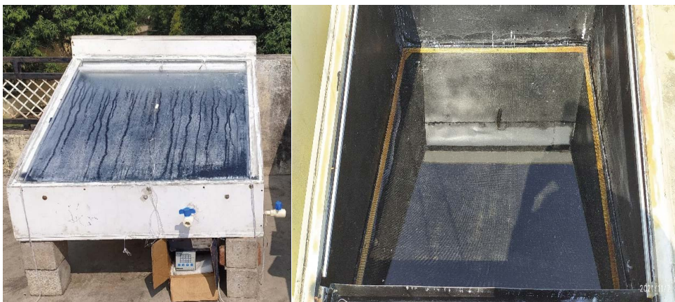
Fig. 1. Conventional solar still setup and wire mesh placement in the basin.
