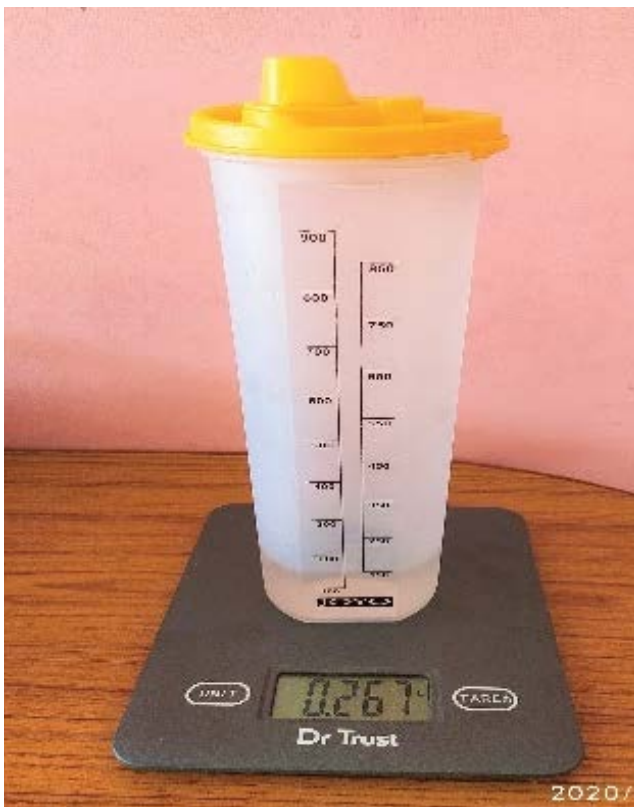
Fig. 4. Weighing machine for measuring distillate yield.
