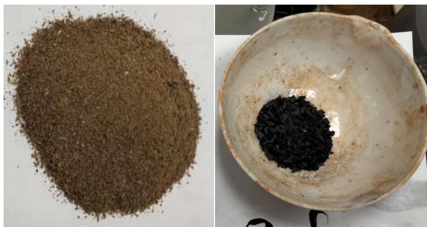
Fig. 1. (a) Dried chicken bones at 300°C and (b) chicken bones ashed at 550°C for 30 min (CBA).
