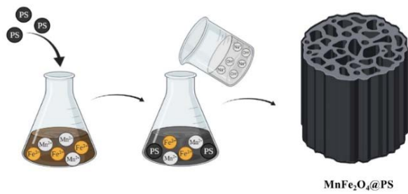
Fig. 1. Synthesis pathway for \text{MnFe}_2\text{O}_4@\text{PS} composites.
