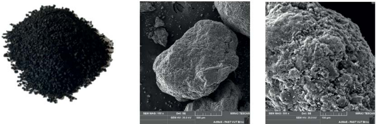
Fig. 2. Filtrasorb F400 sorption material in the original size and in microscopic enlargement.
