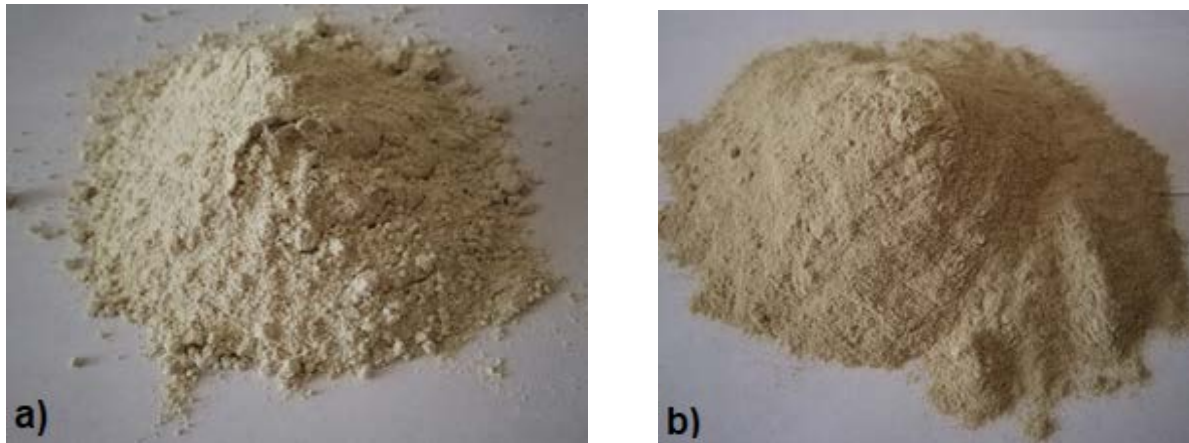
Fig. 3. (a) Dispersed, thermally activated limestone and (b) natural limestone.
