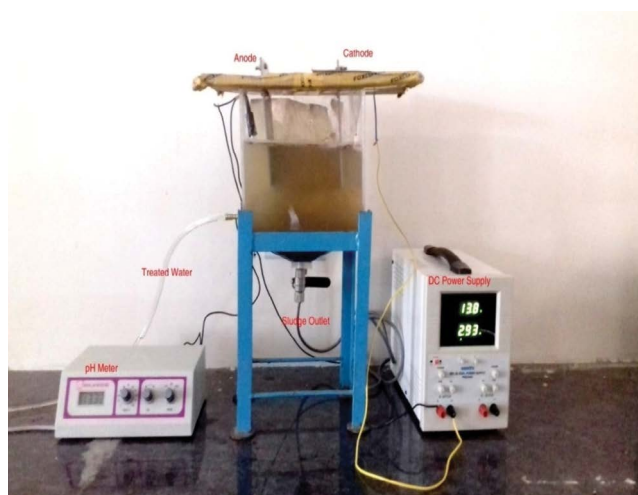
Fig. 1. Photograph view of electrochemical peroxidation reactor.
