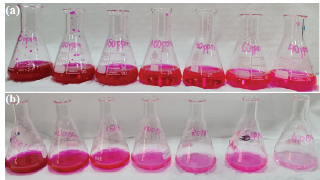
Fig. S3. (a) RhB aqueous solution before adsorption and (b) RhB aqueous solution after adsorption onto the fabricated nano-activated charcoal incorporated sodium alginate-based cross-linked membrane.
