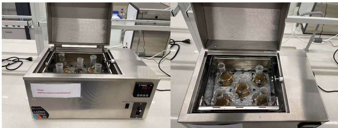
Fig. 1. Test stand – shaking water bath.
