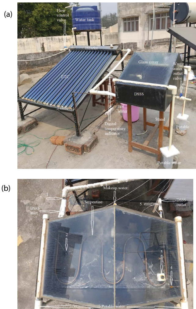
Fig. 1. (a) Evacuated tube collector integrated double slope solar still experimental set-up. (b) Top view of double slope solar still.
