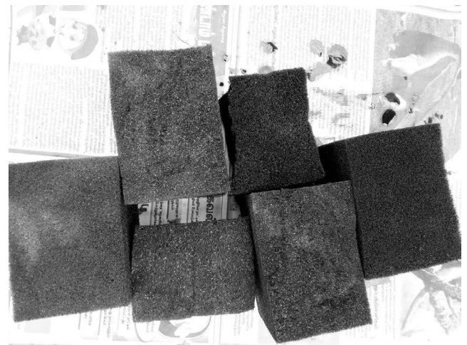
Fig. 2. Photo of the black-painted wick materials used in the CSS basin.
