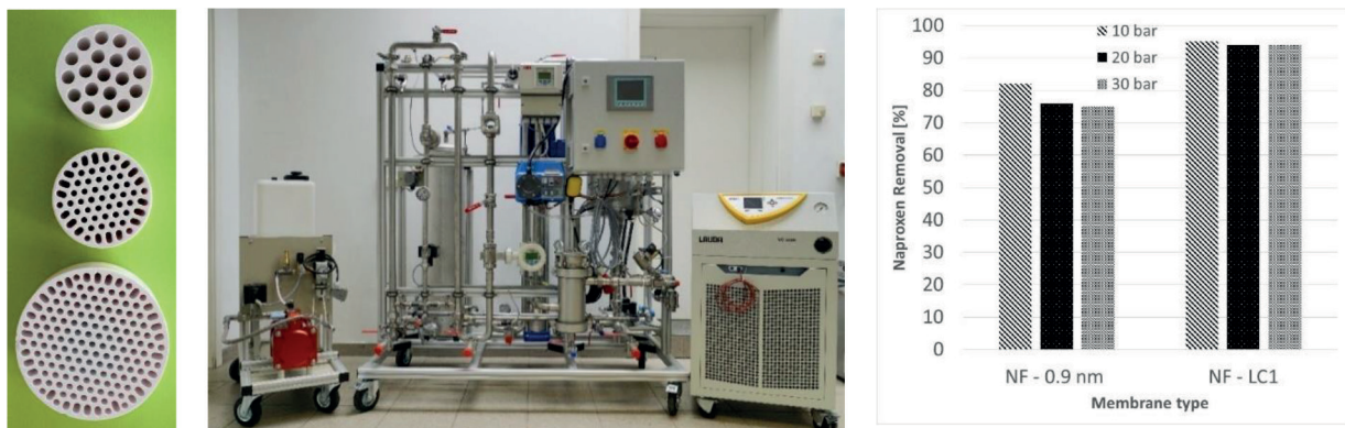
Fig. 1. From left to right: Tubular ceramic nanofiltration membranes of different geometry, IKTS mobile pilot filtration system, retention of painkiller Naproxen by ceramic nanofiltration membrane
