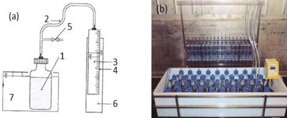
Fig. 2. (a) The anaerobic digester: 1: glass bottle 1 L; 2: connection pipe; 3: gas column; 4: ruler; 5: valve; 6: saturated brine tank; 7: tray and (b) the anaerobic digestion system.
