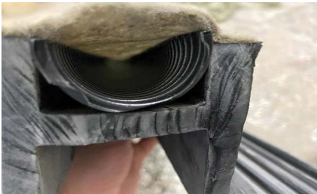
Fig. 8. Schematic diagram of the novel water stop belt structure.
