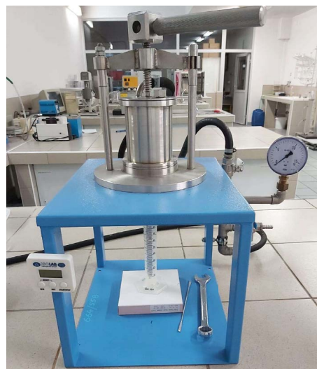
Fig. 2. Pressure filtration station.
